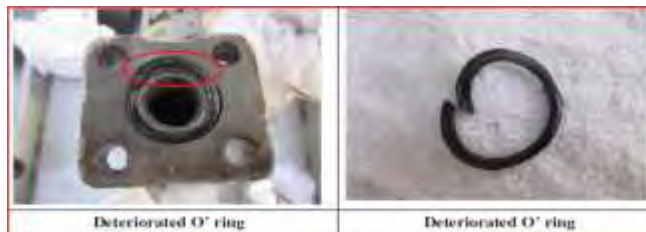
Deteriorated O' ring
